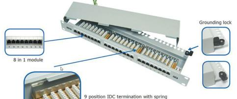
9 position IDC termination with spring wire/contact blades and includes the ninth slot for the drain wire.
